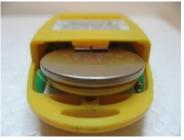
4. Insert new battery, 5. Push battery positive (+) side facing up.
